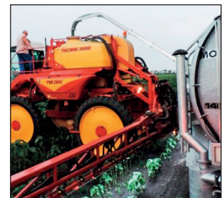
Filling arm up to 4.9 m above the ground.
